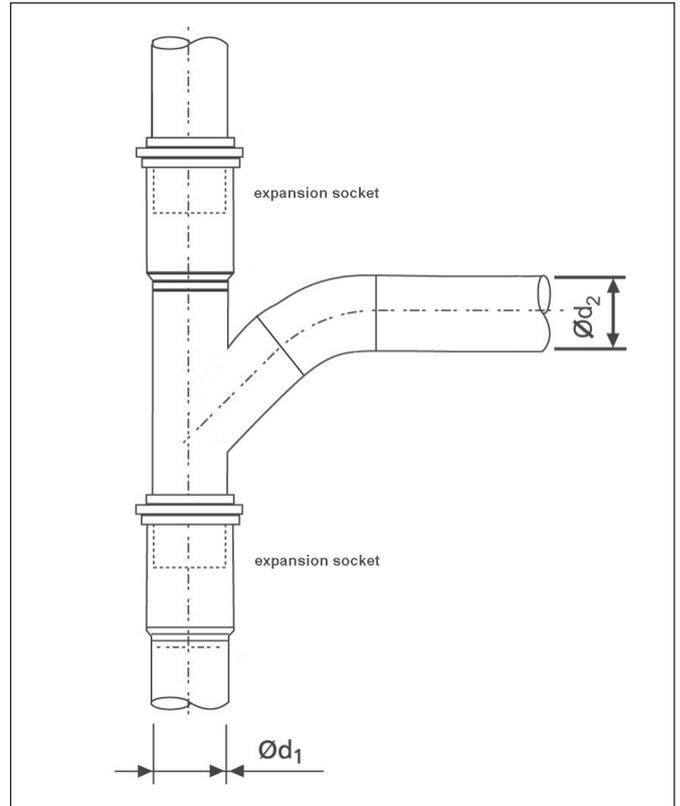
Illustration 4.11 Anchor point with (snap) expansion sockets
