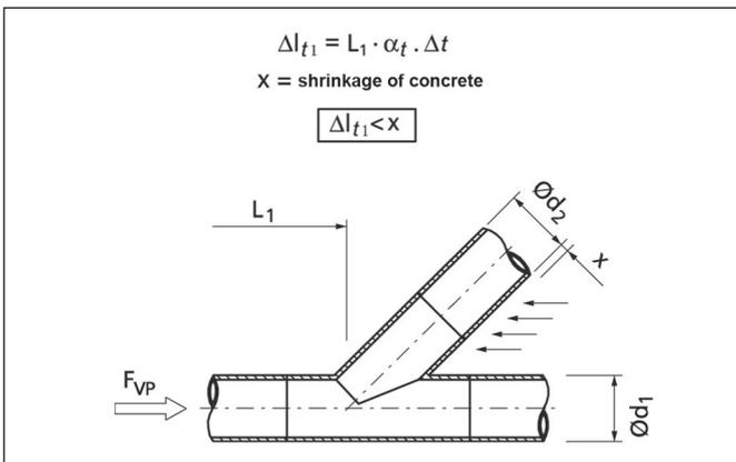
Illustration 4.10 Anchor point with an electrofusion coupler
