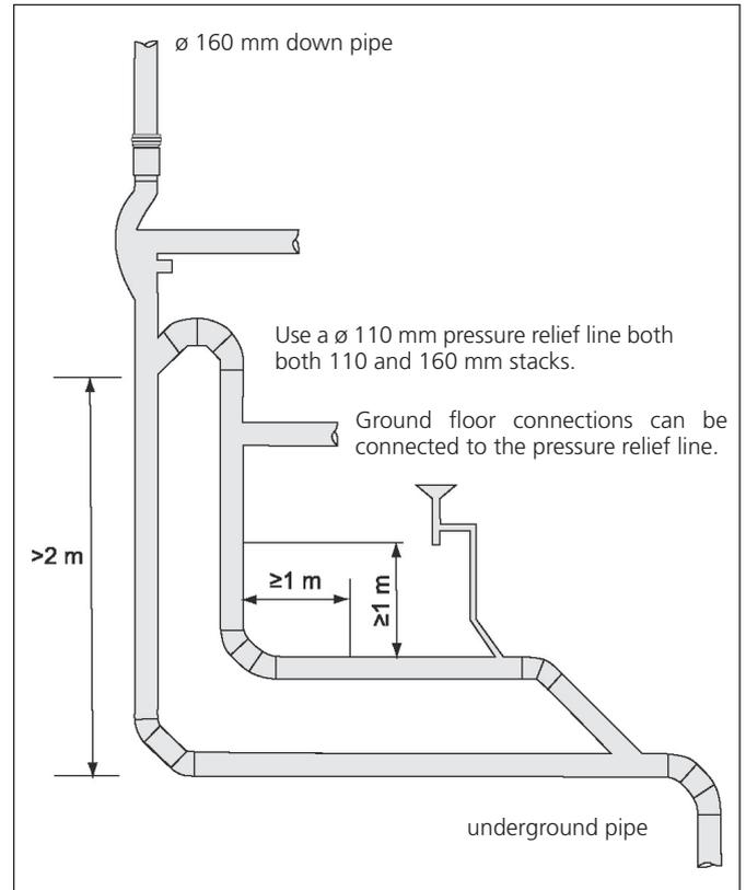
Illustration 5.9 End of the Stack-aerator down pipe
