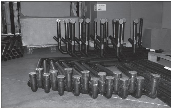
Illustration 9.1 Prefabricated pipe sections
